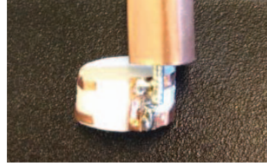
Fig. 2. The fabricated prototype of the circular-shaped balanced inverted-A antenna. The connected coaxial cable and balun are seen at the top.
