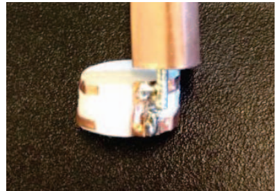
Fig. 4. The fabricated prototype of the circular-shaped balanced inverted-A antenna. The connected coaxial cable and balun are seen at the top.
