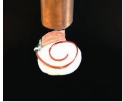
Fig. 1. The fabricated prototype of the spiral monopole antenna. The connected coaxial cable and balun are seen at the top.
